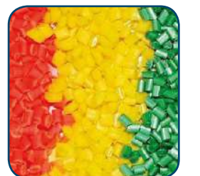
IALA specifications: Pigments integrated into the polyethylene for no painting ever
